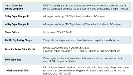
keeps the printer secure yet swivels for ease of motion
