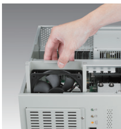
Easy-to-maintain cooling fan
