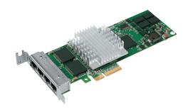
Server Adapter improves performance in multi-processor systems by balancing network loads across multiple central processing units (CPUs). Additionally, the Intel PRO/1000 PT Quad Port LP Server Adapter supports Intel® I/O Acceleration Technology (Intel® I/OAT)² for faster I/O processing on the new Quad-Core and Dual-Core Intel® Xeon® processor-based servers.
