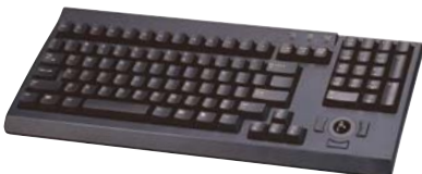
▶ d Compact keyboard integrated with trackball
