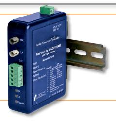
Model FOSTCDRI is Advantech B+B SmartWorx' premium industrial serial to multi-mode fiber optic converter. Its rugged design is UL approved and certified for Class 1/Division 2 industrial environments. It extends data communications up to 4km (2.5 miles). It provides three-way optical isolation on the input, output and power lines.
