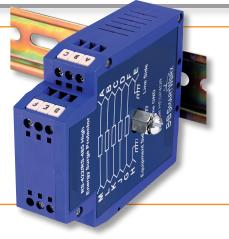
Model HESP4DR meets IEEE 1000-4-5: 1995 and IEEE C62.41-1991 recognized standards for premium surge protectors. It protects against lightning strikes, power surges, and other types of voltage disturbances with three stages of protection for each supported line: a gas discharge tube followed by a series resistor and finally a Transient Voltage Suppresser (TVS). Five RS-422/485 signals on terminal blocks are supported with a
