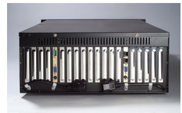
Dual AC power cords for 460W / 570W / 810W redundant power supply
