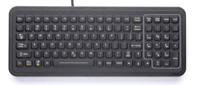
iKey's SlimKey<sup>™</sup> PM-101 panel mount keyboard provides full-sized versatility in a rugged, compact design. When properly installed, the PM-101 is engineered for NEMA 4X protaction from dust, water and corrosive liquids. It is designed for easy integration into workstations, kiosks and industrial environments. The large numeric pad on the PM-101 allows for easy data entry, while the robust polycarbonate case stands up in the roughest of conditions.
