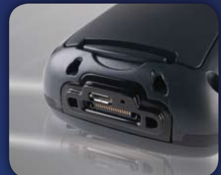
USB-on-the-Go for sending and receiving data, setting automatically the behavior of the PDA
