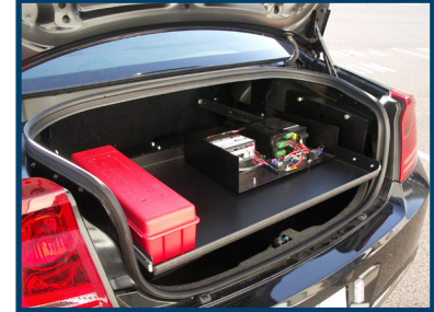
Tray slides out for easy access to equipment. (C-TTB-CHGR shown)
