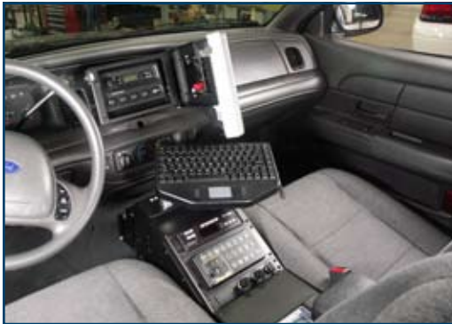
Crown Victoria Swing Out Mount with a Datalux Computer (C-DMM-101, C-MM-205)
