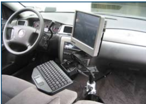
Universal Monitor and Keyboard Pole Mount with Data911 Computer (C-MKM-101, C-MM-204)
