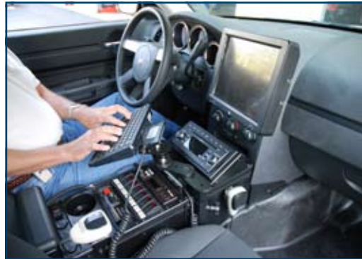
Dodge Charger Tilt Swivel Mount with a L3-MV2 Computer (C-DMM-104, C-MM-201, C-MM-302)
