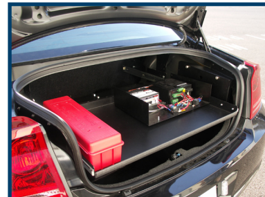
Tray slides out for easy access to equipment. (C-TTB-CHGR shown)
