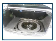
Premium Fold Down Trunk Tray assembly with slide out equipment tray allows easy mounting and access to electronic components without blocking the spare tire.
