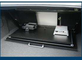
Havis Fold Down Trunk Trays mount cleanly inside the vehicle without drilling holes.
