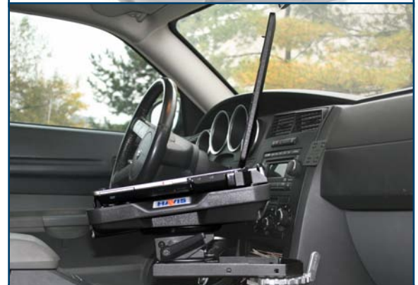
Top: Macro Alignment Bracket ensures proper docking.
