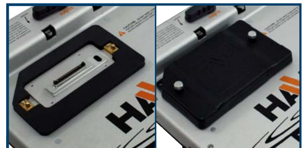
Docking Connector Gasket (Left) ensures water and dust protection while computer is docked. Docking Connector Cover (Right) protects Connector while computer is not docked.
