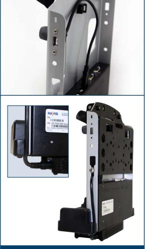
Top: Integrated Remote USB Extension Cable for USB access from either or both sides of Docking Station. Bottom: Integrated power supply cord routed for secure connection and ease of mounting. (DS-PAN-602 shown)
