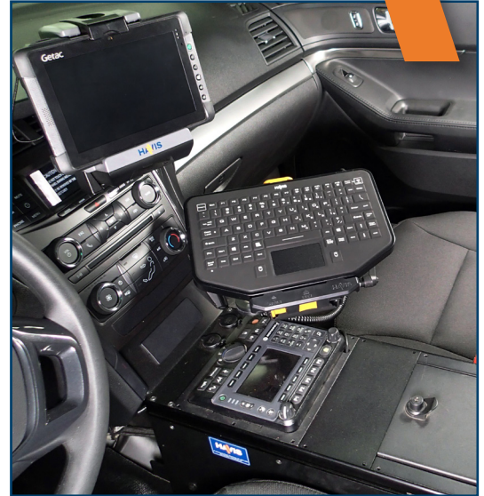
One touch button illuminates red monochrome backlight
