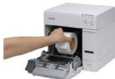
Open cover, drop in paper roll, close cover! That easy is the paper load for the TM-C3400
