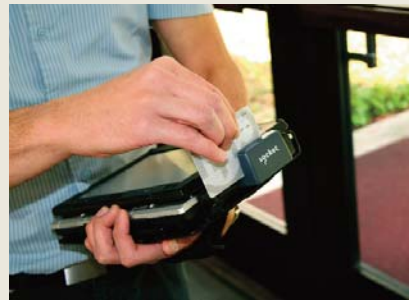
CF Mag Stripe Reader Card in a tablet computer
