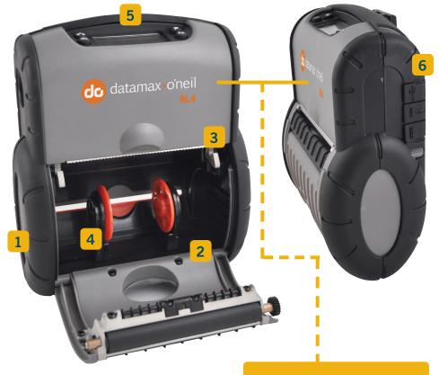
**6** Port covers are made of a durable, rubberized material to protect against external environmental agents when ports are not in use.
