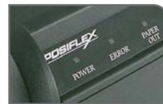
Three LED colour indicators for status display.
